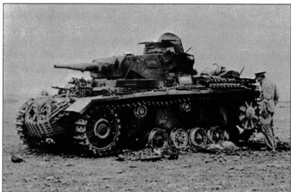
The Panzer III fared very badly in its first encounters with the British Matilda. Prodigious efforts to increase their protection with bogies and track links did not save this crew, apparently. (Imperial War Museum)
