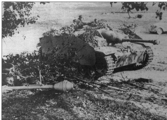
Later models of the StuG were armed with a high-velocity gun; this type of mantlet was known as a Saukopf (pig's head). The vehicle has also been fitted with side skirts as a defence against hollow-charge weapons such as that held by the infantryman in the foreground. (Bundesarchiv)
