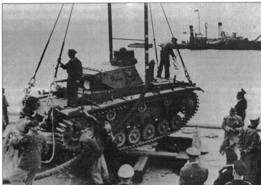
The Tauchpanzer , or Diving Tank, seen here during trials for Operation 'Sea Lion'. Vehicles of this type were used successfully in the crossing of the River Bug during the initial stages of 'Barbarossa' in June 1941. (Bundesarchiv)
